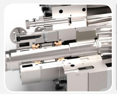
The standard double mechanical seal can be used for pressures from vacuum up to 15 bar (210 psig). The seal can handle viscosities from 0,2 up to 1.000.000 cp (mPas). Maximum temperature of the liquid is about 300°C. For higher pressures and temperatures special designs exist.
