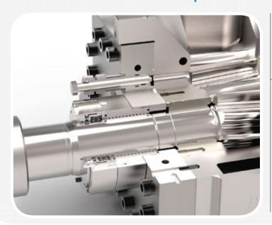
As an alternative, the vacuum viscoseal can also be combined with a lip seal instead of a stuffing box. The buffer fluid of this static shaft seal acts as barrier. If the pump is stopped for a short time this design prevents air getting sucked in the pump through the shaft seal.
